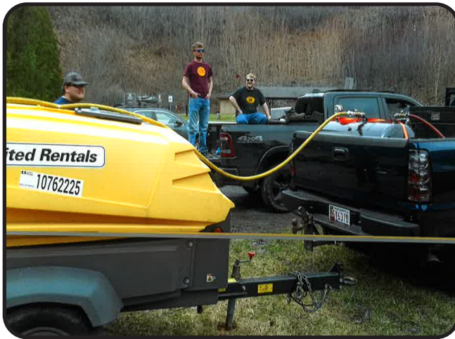
A truck with just an air tank is getting refilled between runs with the portable air compressor.
