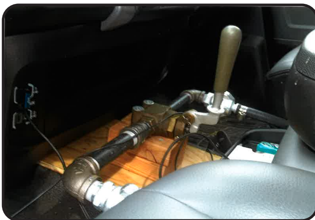
The control handle built into the cab of the truck for regulating the air flow to the horns.
